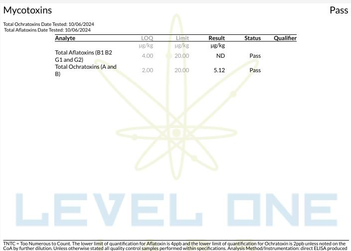
CoA by further dilution. Unless otherwise stated all quality control samples performed within specifications. Analysis Method/Instrumentation: direct ELISA produced by Romer Labs and read on Bio-Tek 800TS microplate reader. Procedure followed SOP-LM-018. Methods used per AZDHS R9-17-404.03 and R9-17-404.04 and limits set by AZDHS R9-17 Table 3.1. ADHS approved method.
